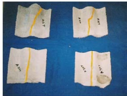
Fig. 4: Fractured Specimens of Corrugations After the Splitting Test due to Impact Loads ( V_f = 1.0\% ; Fly ash = 0 - 30%)
