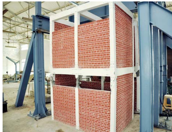
Figure-9. Test structure (1) with failure in the bottom and drift of the top storey (Constructed at VLBJCET, Coimbatore).
