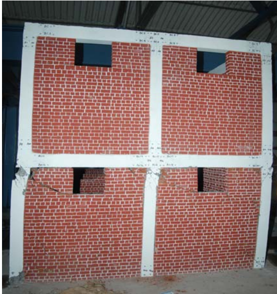
Figure-10. Test structure-2 with failure in the bottom and drift of the top storey (Constructed at VLBJCET, Coimbatore).
