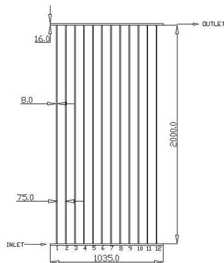
**Figure-3.** Sectional view of 12 numbers riser tubes flat plate collector.
