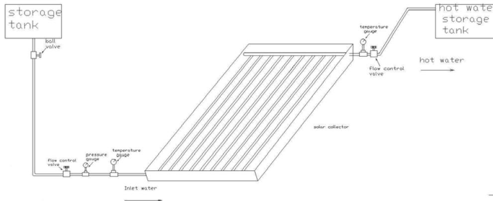
**Figure-1.** The schematic diagram of flat-plate collector solar water heater.
