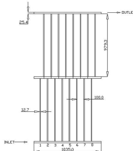
**Figure-4.** Sectional view of Zig-Zag arrangement of riser tubes.
