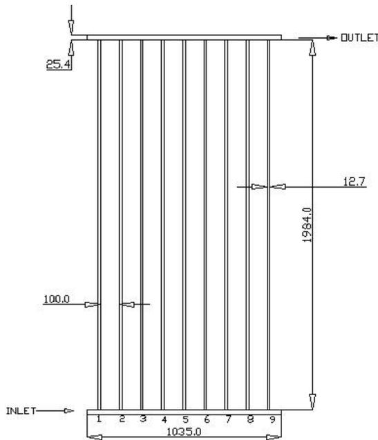
**Figure-2.** Sectional view of 9 riser tubes flat plate collector.
