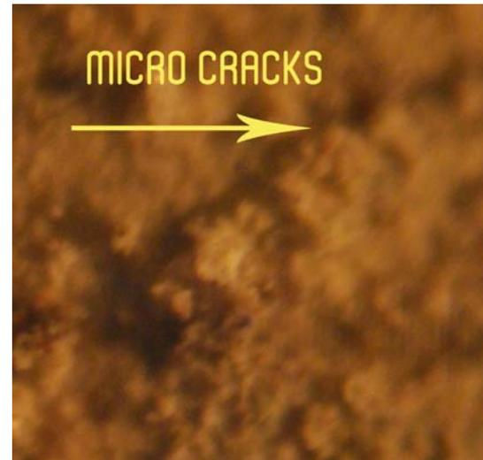
**Figure-8.** Microscope study of concrete sample (RAC+10F) after heating at 800°C.
