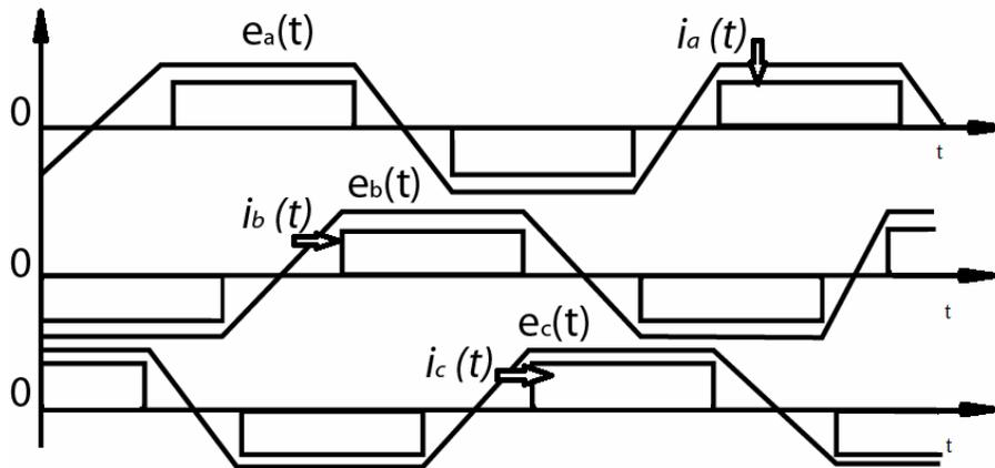
Figure-1. Typical waveforms of the back emfs and the corresponding stator currents of a PMBLDC motor.
