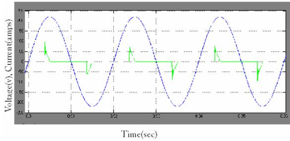
Figure-4. Input voltage and current (PF=0.98)
