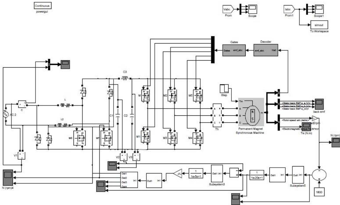
Figure-10. Closed loop speed control of PMBLDC motor with PFC half bridge converter.
