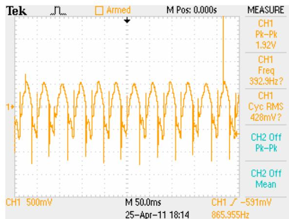
Figure-14(d-i). Terminal voltages of motor.
