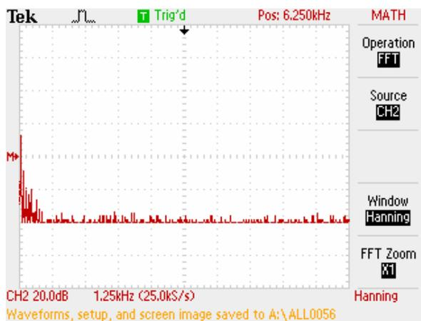
Figure-14(g). Harmonic spectrum of motor current.
