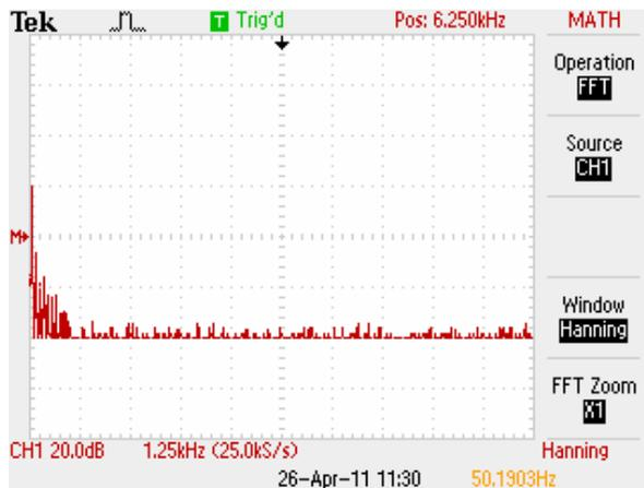
Figure-14(f). Harmonic spectrum of motor voltage.
