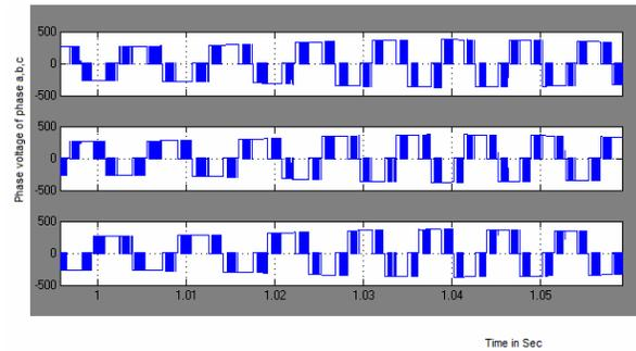
Figure-5. Phase voltage supplied to the stator windings.
