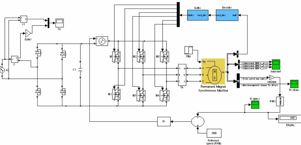
Figure-3. Closed loop model of PMBLDC motor.
