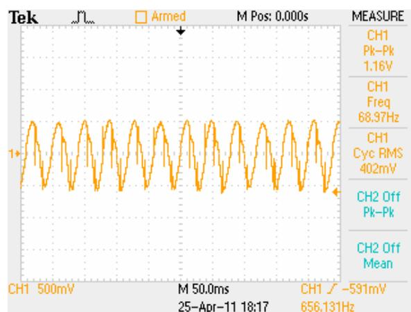
Figure-14(d-ii). Terminal voltages of motor.
