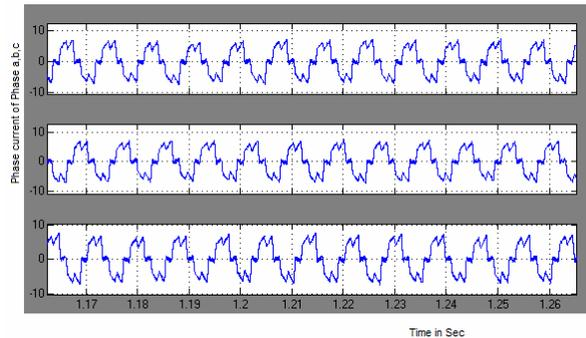
Figure-6. Three phase inverter stator current.
