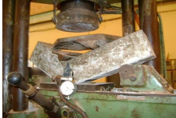
Figure-7. Flexural test result.
