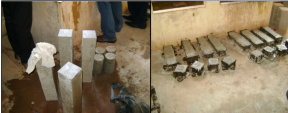
Figure-5. Concrete cubes, beams and cylinder samples.
