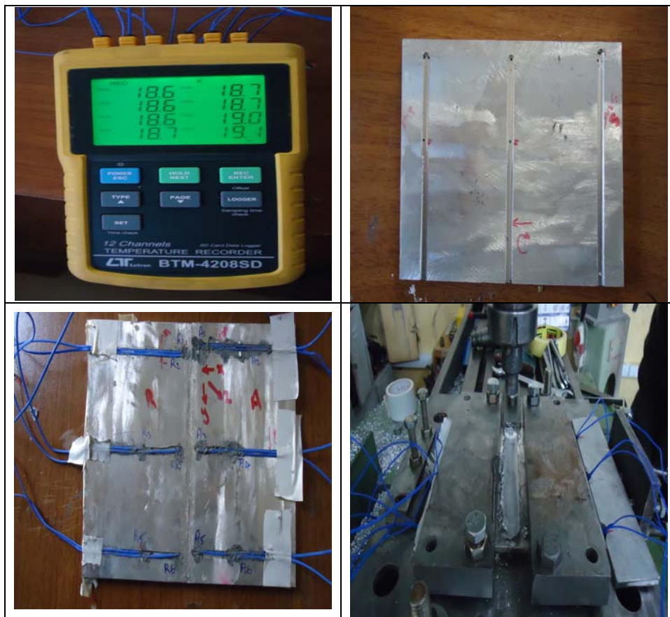
Figure-4. Temperature recorder and hole drill thermocouple position on workpiece.
