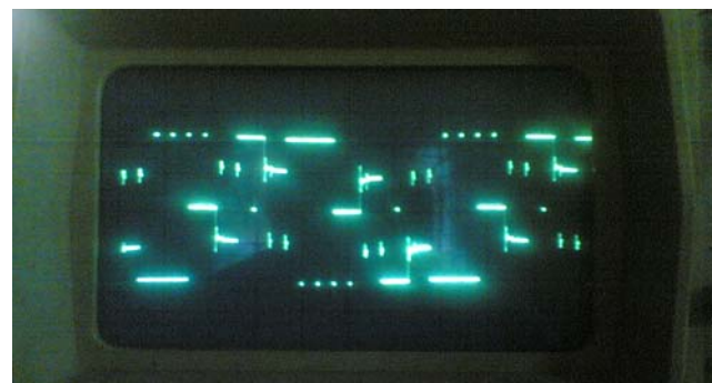
Figure-3c. Line voltage with motor load.
