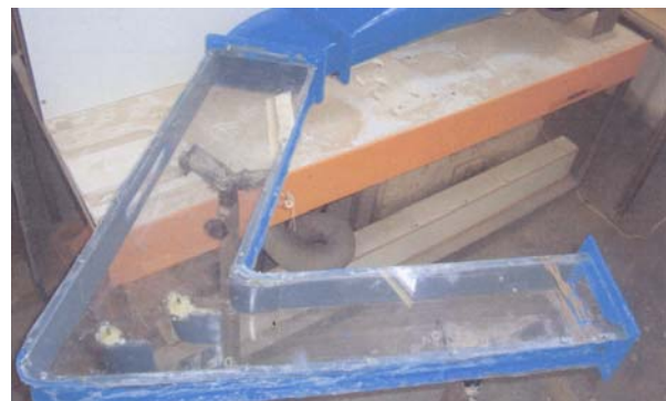
Figure-4. Blade row attached to one side of end wall.
