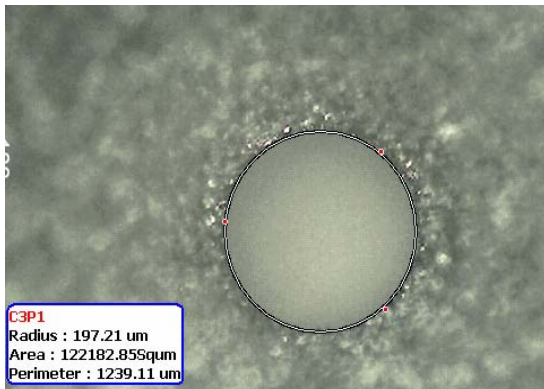
Figure-3. Optical Microscope image of micro hole machined in 9 th experiment.
