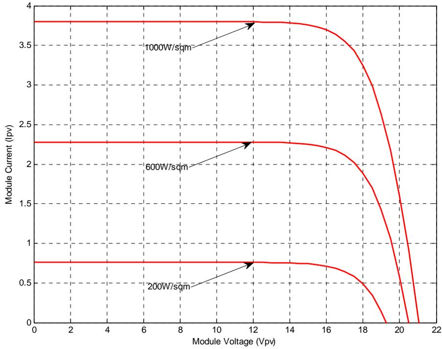
Figure-10. I-V characteristic-varying irradiance- constant temperature.
