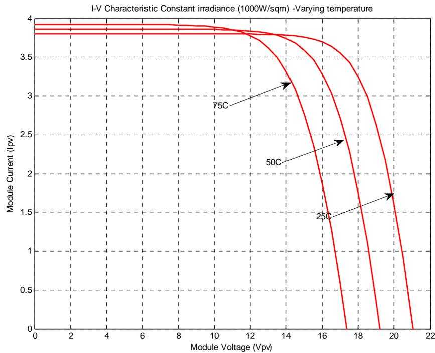
**Figure-12.** I-V characteristic-constant irradiance (1000W/sqm)-varying temperature.
