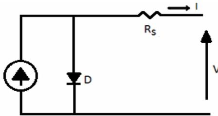
Figure-1. Solar cell model using single diode
