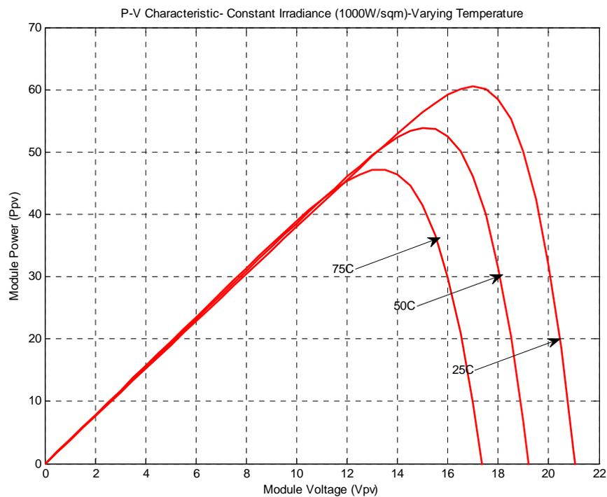
**Figure-13.** P-V characteristic-constant irradiance (1000W/sqm) varying temperature.
