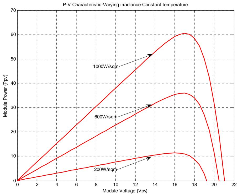
Figure-11. P-V characteristic-varying irradiance-constant temperature.
