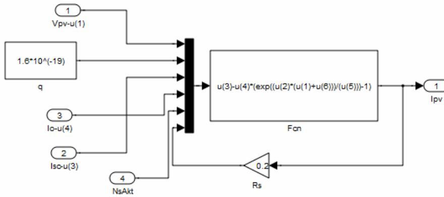
**Figure-7.** This model executes the function given by equation 8.
