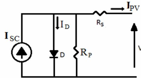
Figure-2. Solar cell model using single diode with  $R_S$  and  $R_P$ .
