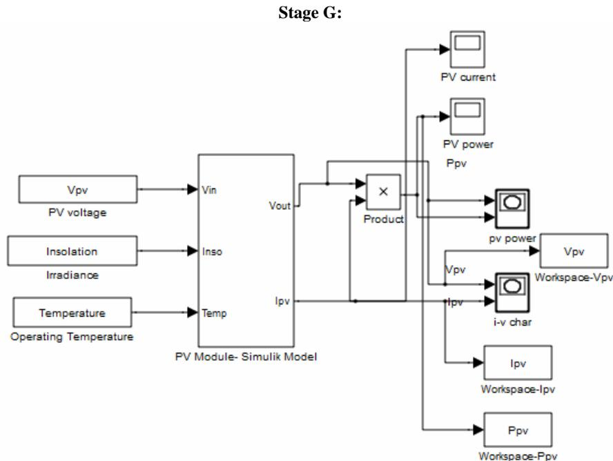
**Figure-9.** This is the final model which takes irradiation, operating temperature and Module voltage as input and gives the output current  $I_{PV}$  and output voltage  $V_{PV}$ .
