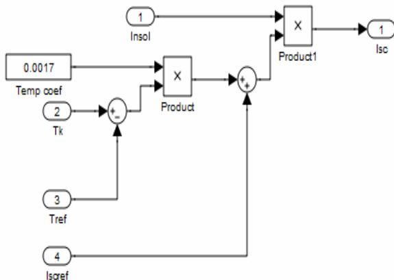
**Figure-3.** This model calculates the short circuit current  $I_{sc}$  at given operating temperature.
