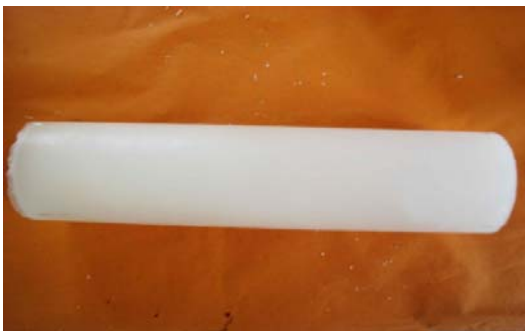
Figure-1. Prepared paraffin wax fuel grain.
