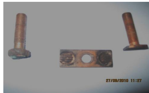
Figure-5. Pitting in the solenoid contacts.
