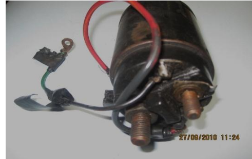
Figure-4. Damaged solenoid terminal.
