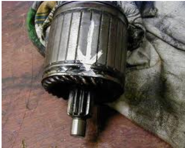
Figure-8. Starter motor armature fault.
