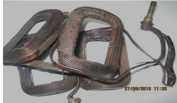
Figure-9. Damaged field winding.
