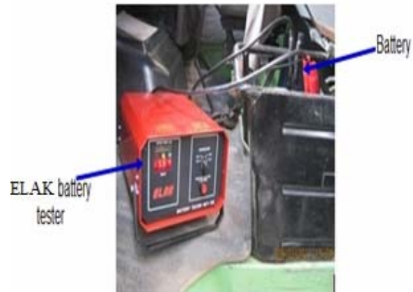
Figure-16. Battery tester to measure voltage dip during cranking.
