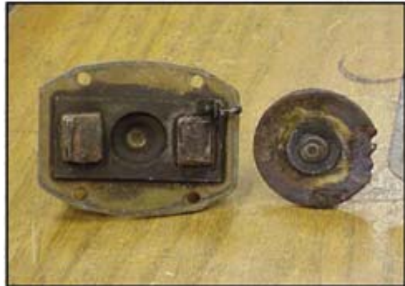
Figure-8. Damage caused by low system voltage.
