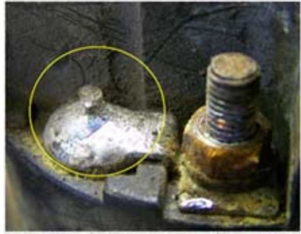
Figure-7. Good solder on solenoid.
