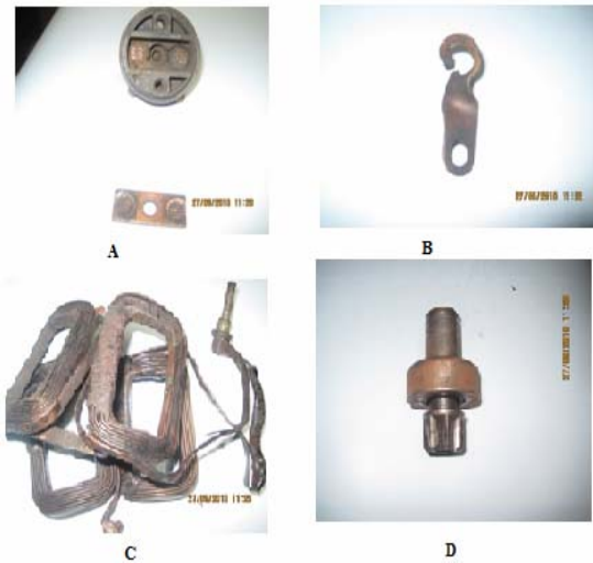
Figure-5. A. Solenoid contact arcing (pitting) fault. B. Motor to solenoid connector warp C. Field Winding fault. D. Pinion teeth fault
