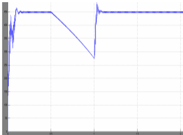
Figure-3. DC link capacitor voltage of Vienna rectifier.
