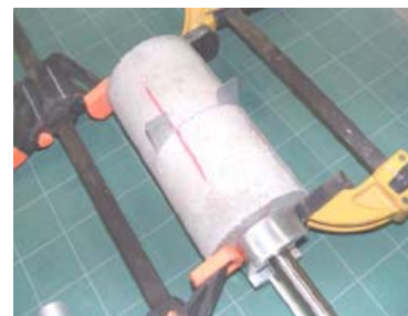
Figure-8. Artificial crack making.
