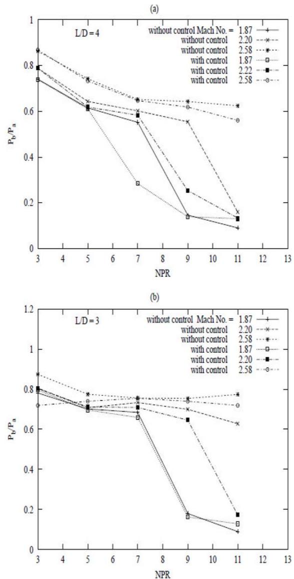
Figure-5. Base pressure variation with NPR.
