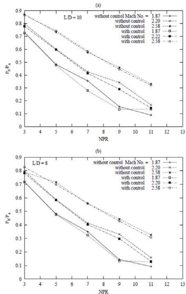
**Figure-3.** Base pressure variation with NPR.
