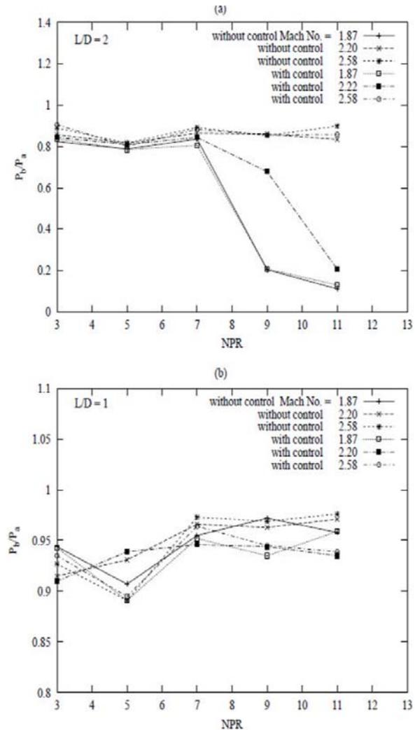
Figure-6. Base pressure variation with NPR.
