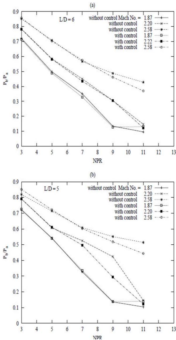
Figure-4. Base pressure variation with NPR.
