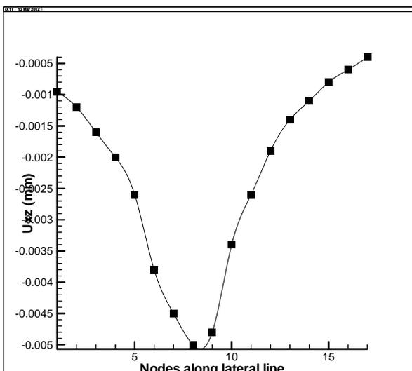
Figure-14. Deformation in (x and z) direction.
