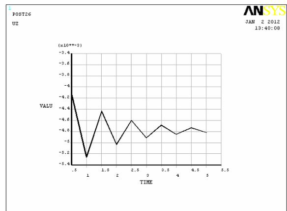
Figure-17. Dynamic stress of Uz when damping coefficient = 0.04.
