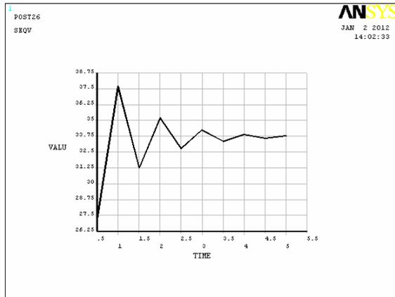
**Figure-24.** Dynamic stress of Von misses when damping coefficient = 0.06.
