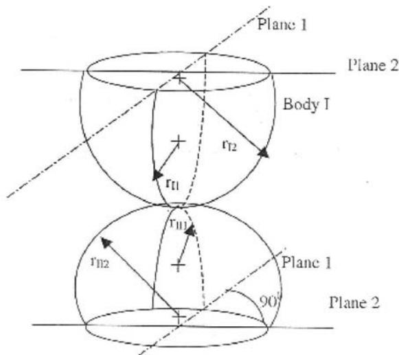
**Figure-3.** Geometry of contacting bodies.
