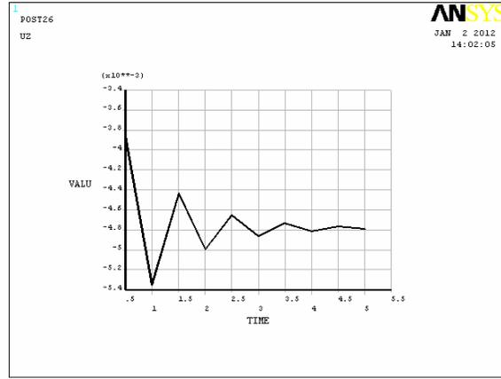
Figure-23. Dynamic stress of Uz when damping coefficient = 0.06.
