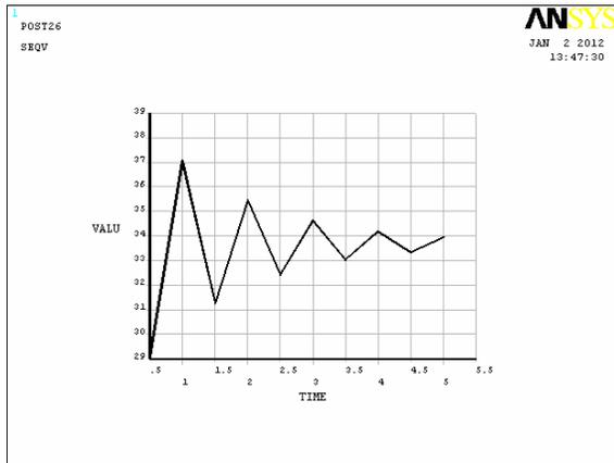
Figure-18. Dynamic stress of Von misses when damping coefficient = 0.04.
