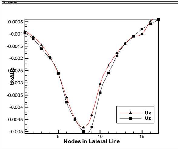
Figure-13. Comparison deformation in (x and z) direction.
