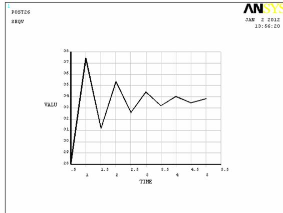
Figure-21. Dynamic stress of Von misses when damping coefficient = 0.05.
