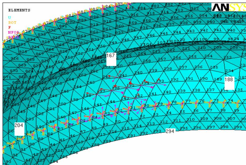
Figure-5. Nodes along line of load effect and surface of raceway groove.
