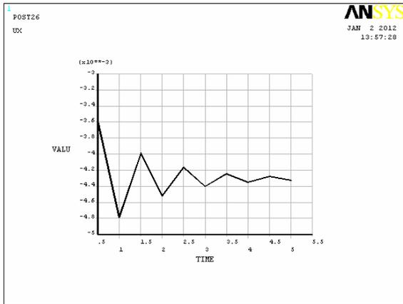
Figure-19. Dynamic stress of Ux when damping coefficient = 0.05.
