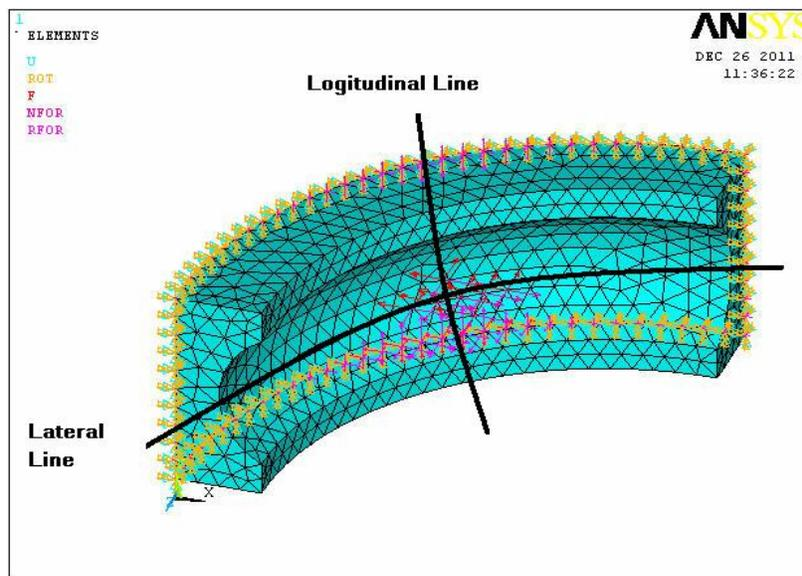
Figure-4. Geometry of outer race section.
