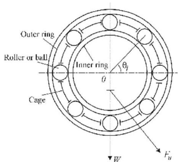
**Figure-2.** A schematic diagram of a rolling element bearing.
