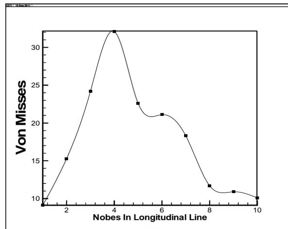
Figure-10. Von Misses in longitudinal line.
