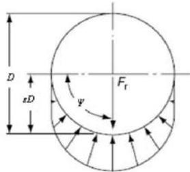
**Figure-1.** The load distribution in a bearing under radial load.
