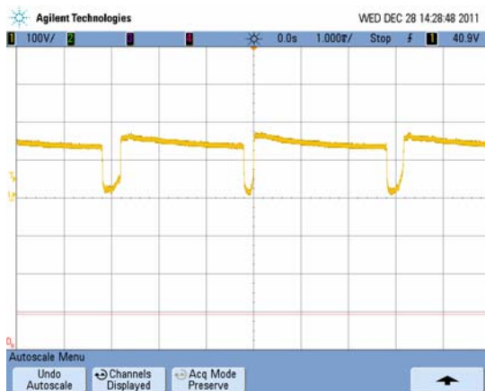
Figure-11. Experimental voltage waveform recorded for a cable length 15m at the inverter output terminals.
