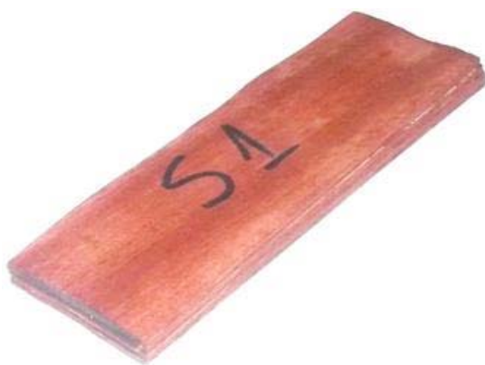
(a) Specimen of Sapelli LVL lumber S1
