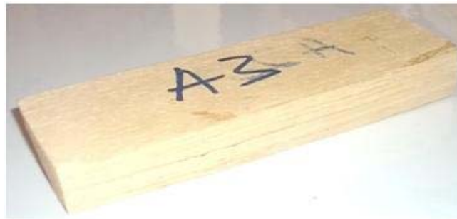
(c) Specimen of Ayous LVL lumber A3.
