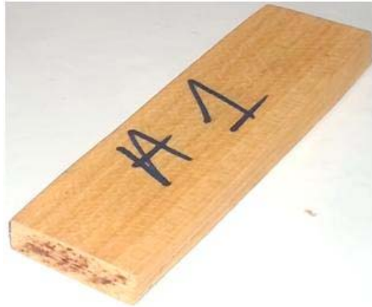
(a) Specimen of Ayous LVL lumber A1.
