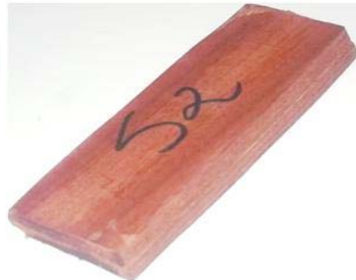
(b) Specimen of Sapelli LVL lumber S2
