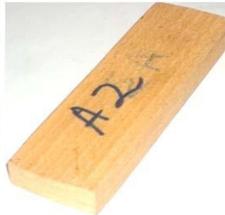
(b) Specimen of Ayous LVL lumber A2.
