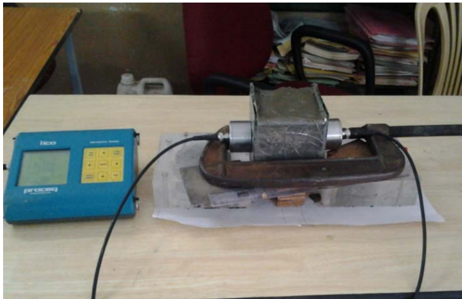
Figure-1. Experimental test setup showing the ultrasonic pulse velocity measurements.
