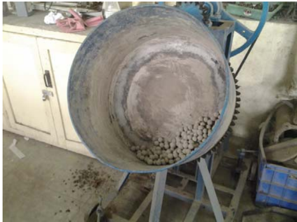
Figure-1. Fabricated disc pelletizer machine.
