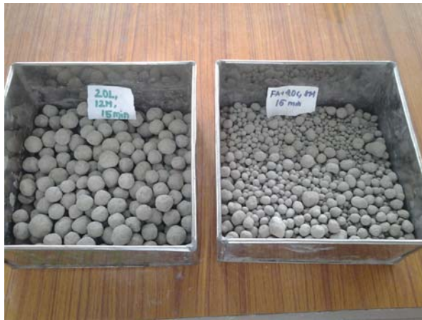
Figure-3. Pelletized fly ash aggregate for 15 minutes duration.
