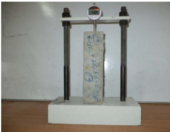
**Figure-1.** Typical picture showing for digital length comparator.
