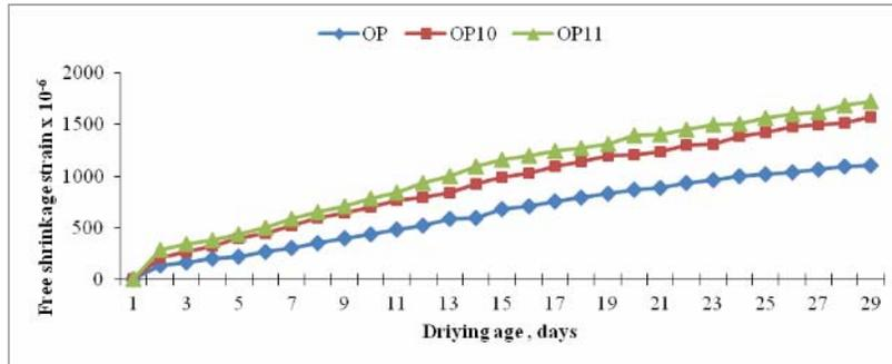
Figure-6. Drying shrinkage results for concrete containing OPC and various dosage of accelerator and steel fibre at 28 days.
