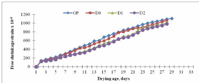
**Figure-11.** Drying shrinkage results for concrete containing OPC and various level of flyash, accelerator and steel fibre at 28 days.
