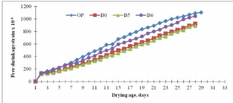
**Figure-10.** Drying shrinkage results for concrete containing OPC and various level of flyash, accelerator and steel fibre at 28 days.
