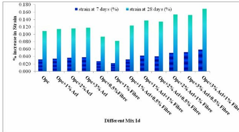
**Figure-14.** Variation of shrinkage strain for different concrete mixes containing OPC with dosages of accelerator and steel fibre.
