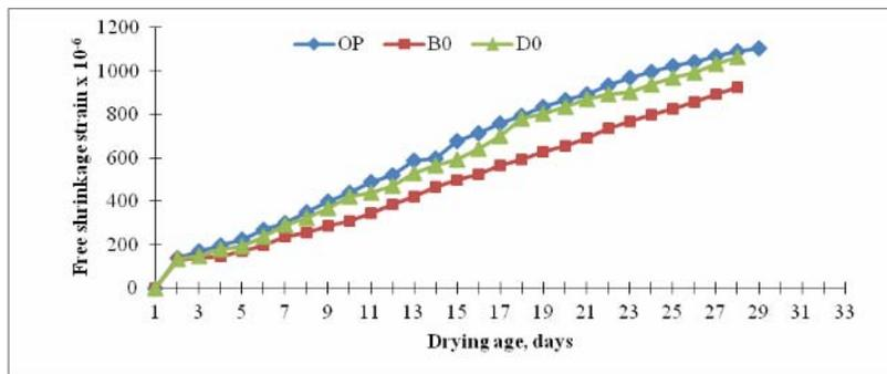
Figure-7. Drying shrinkage results for concrete containing OPC and various level of flyash at 28 days.
