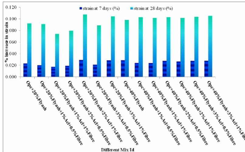
**Figure-15.** Variation of shrinkage strain for different concrete mixes containing OPC, flyash, accelerator and steel fibre.
