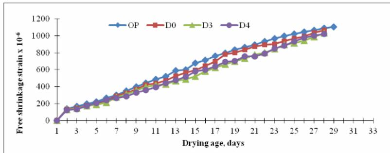
**Figure-12.** Drying shrinkage results for concrete containing OPC and various level of flyash, accelerator and steel fibre at 28 days.
