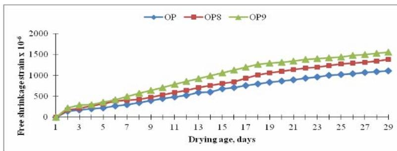
Figure-5. Drying shrinkage results for concrete containing OPC and various dosage of accelerator and steel fibre at 28 days.
