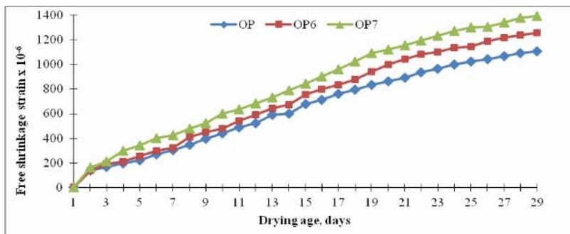
Figure-4. Drying shrinkage results for concrete containing OPC and various dosage of accelerator and steel fibre at 28 days.
