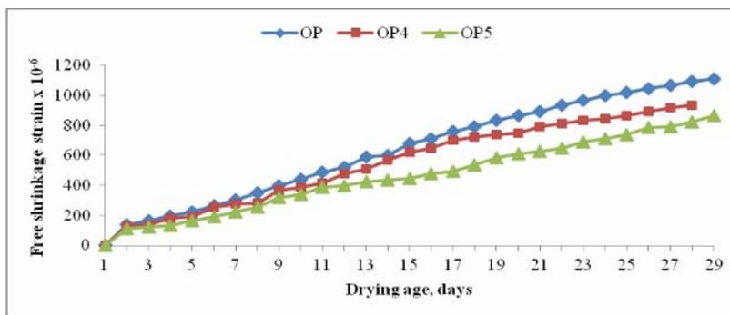
Figure-3. Drying shrinkage results for concrete containing OPC and various dosage of steel fibre at 28 days
