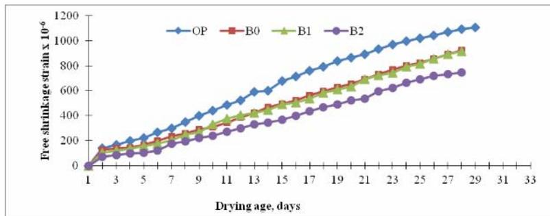
Figure-8. Drying shrinkage results for concrete containing OPC and various level of flyash, accelerator and steel fibre at 28 days.
