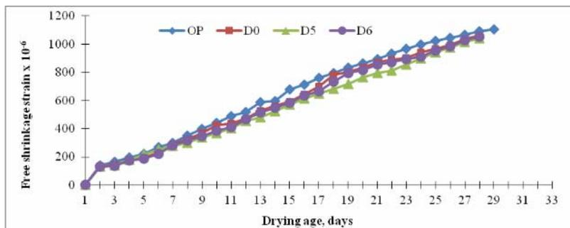
**Figure-13.** Drying shrinkage results for concrete containing OPC and various level of flyash, accelerator and steel fibre at 28 days.
