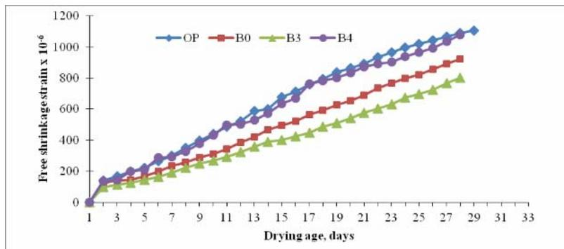
Figure-9. Drying shrinkage results for concrete containing OPC and various level of flyash, accelerator and steel fibre at 28 days.
