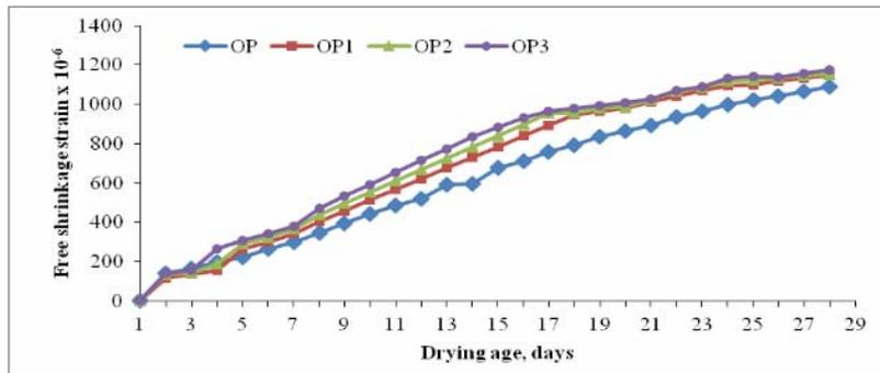
Figure-2. Drying shrinkage results for concrete containing OPC and various dosage of accelerator at 28 days.
