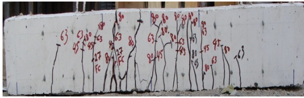
(a). Failure mode for beam ( D_{250}V_0 )
