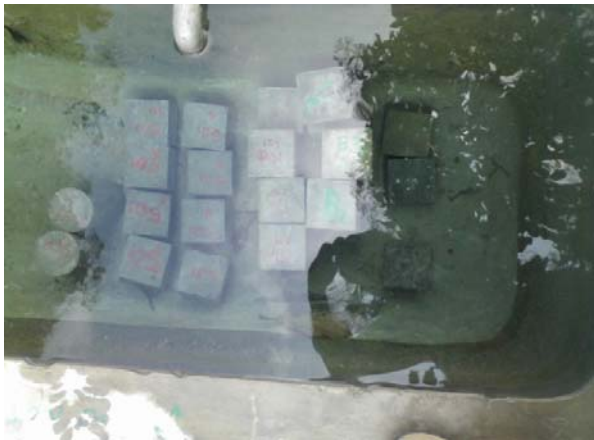
Figure-2. Concrete specimens cured in water.
