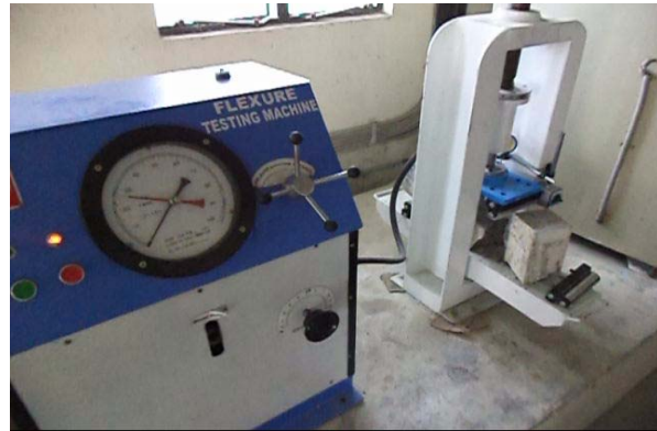
Figure-3. Compression and flexural test setup.
