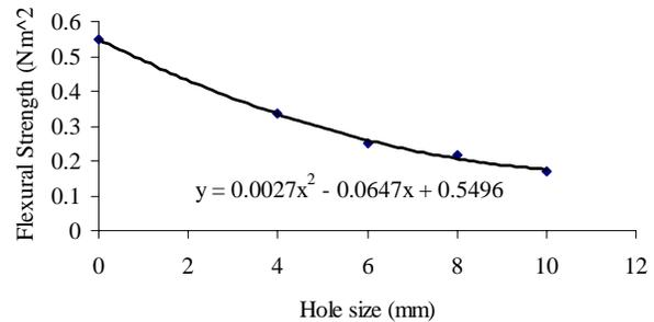
Figure-7. Flexural strength Vs hole size.
