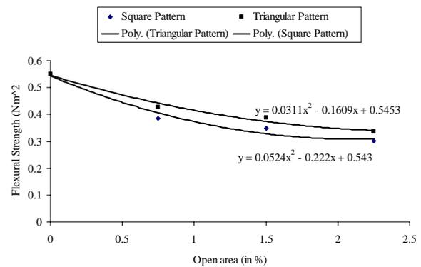
Figure-8. Flexural strength Vs open area (for square and triangular pattern).
