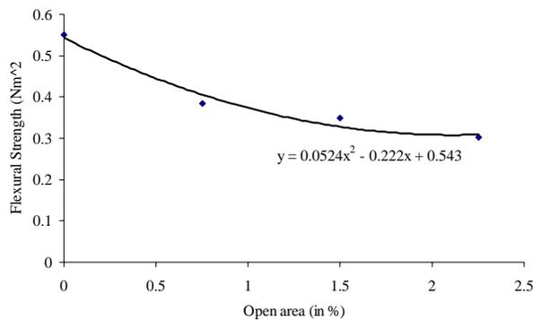
Figure-6. Flexural strength Vs open area.
