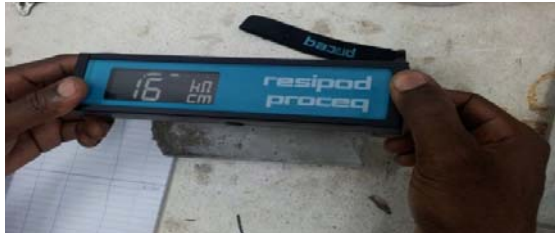
Figure-3. Concrete electrical resistivity measurement.
