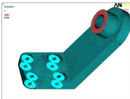
Figure-6. Meshing of third model (engine mount without rib).
