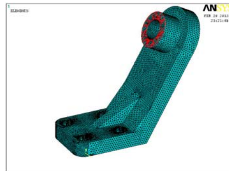
Figure-4. Meshing of second model (engine mount with suggested rib design).
