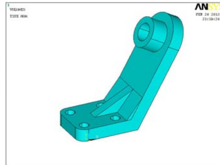
Figure-3. Second model (engine mount with suggested rib design).
