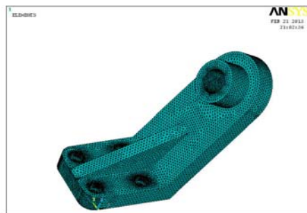
Figure-2. Meshing of first model (engine mount with standard rib design).
