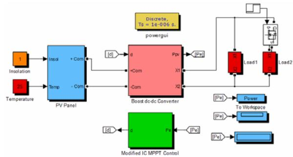
**Figure-9.** MPPT Control PV MATLAB/Simulink model.
