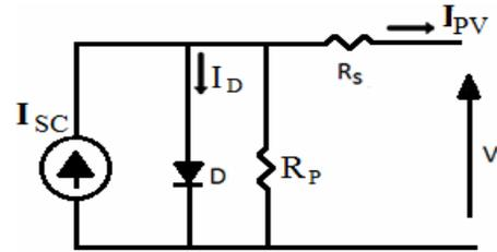
Figure-3. Solar cell model using single diode with  $R_s$  and  $R_p$ .
