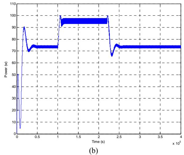
**Figure-10.** Output power of the PV (a) with and (b) Without MPPT under varying load conditions.
