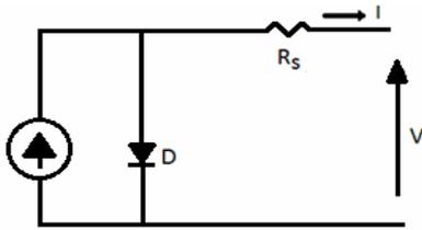
Figure-2. Solar cell model using single diode.
