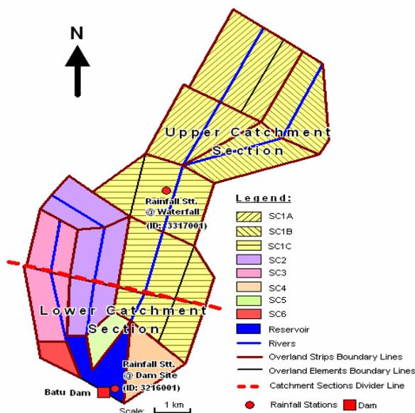
**Figure-4.** Finite element overland strips delimitation.
