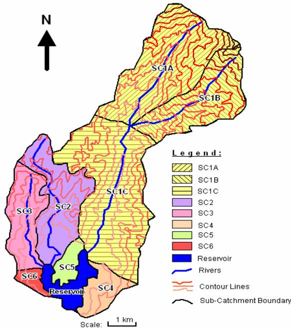
**Figure-3.** Sub-catchments delimitation of Batu dam catchment.
