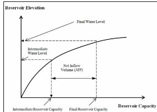
Figure-5. Batu dam reservoir elevation-capacity curve.
