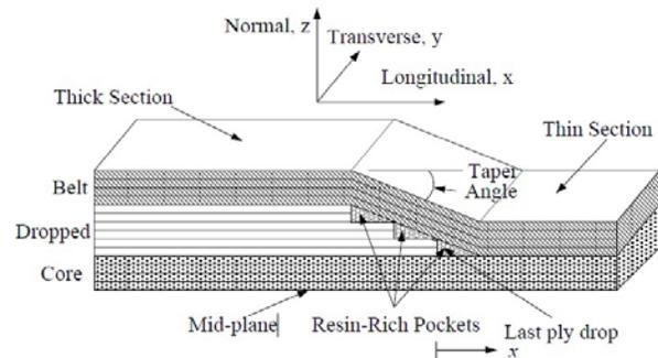
**Figure-1.** Schematic diagram of tapered specimen.
