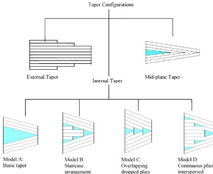
**Figure-2.** Schematic illustration of taper configurations.
