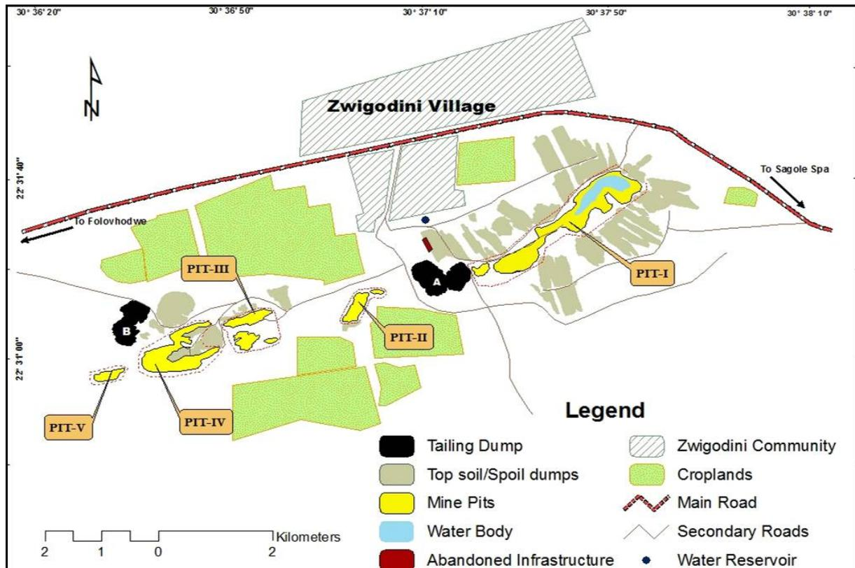
Figure-1. Layout of existing features of abandoned Nyala Mine (from Mhlongo, 2012).
