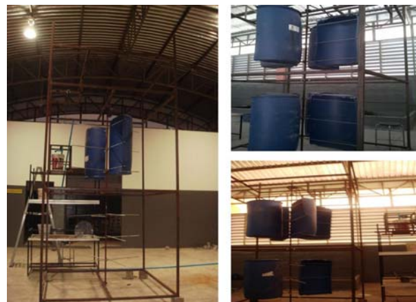
Figure-4. The vertical axis wind turbine was adjusted the number of blades.
