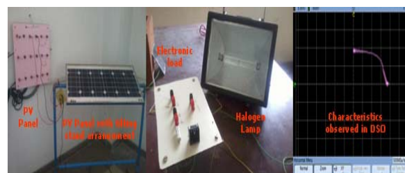
Figure-5. Experimental setup to observe the PV module characteristics
