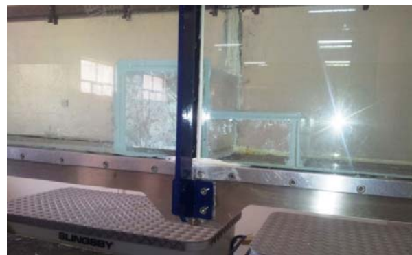
Figure-3. The tested single-step weir.
