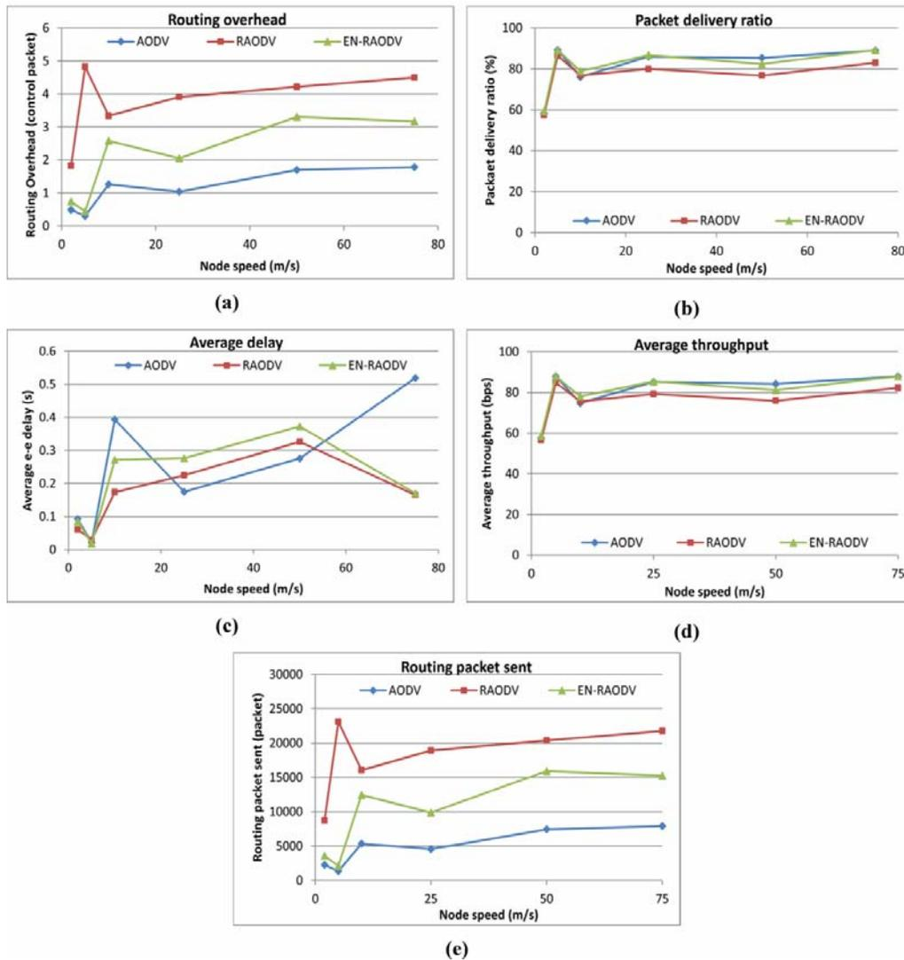
Figure-6. EN-RAODV, RAODV and AODV versus node speed.
