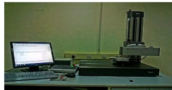
**Figure-3.** Experimental setup for surface roughness measurement.
