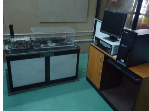
Figure-3. Wear testing machine.
