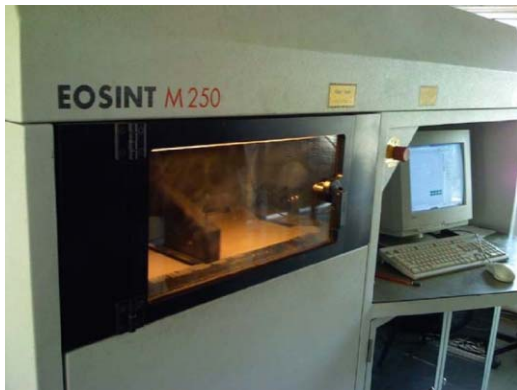
Figure-2. Sintering using DMLS machine.
