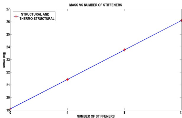
Figure-9. Mass vs. no. of stiffeners.
