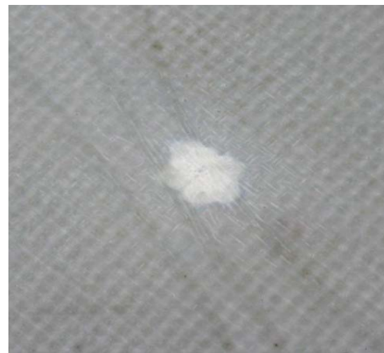
Figure-8. Back damage appearance in laminate 1 at Impact energy of 17.24 J.
