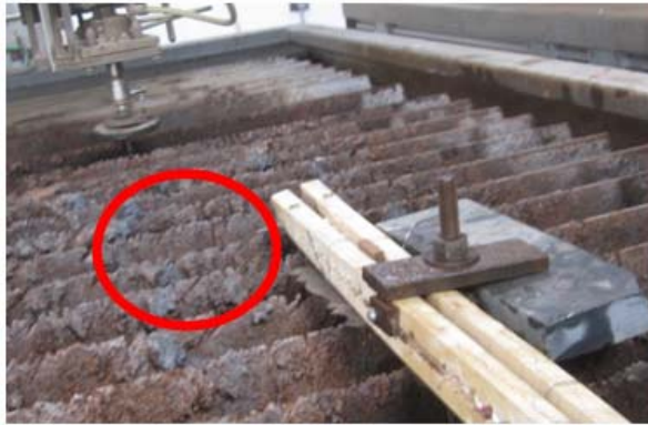
Figure-1. Fixture found perpendicular to the working table.
