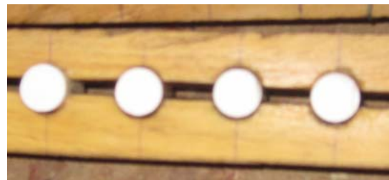
Figure-6. Offset holes to hold pieces of varying diameter.
