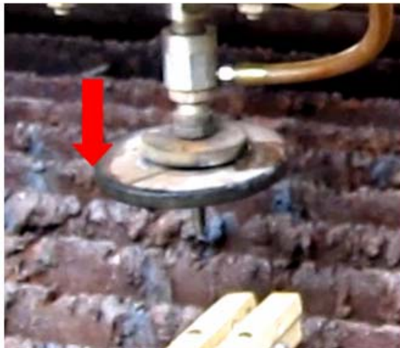
Figure-14. Orientation of nozzle to the work piece.
