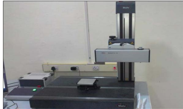
**Figure-1(b).** Set up for surface roughness measurement.
