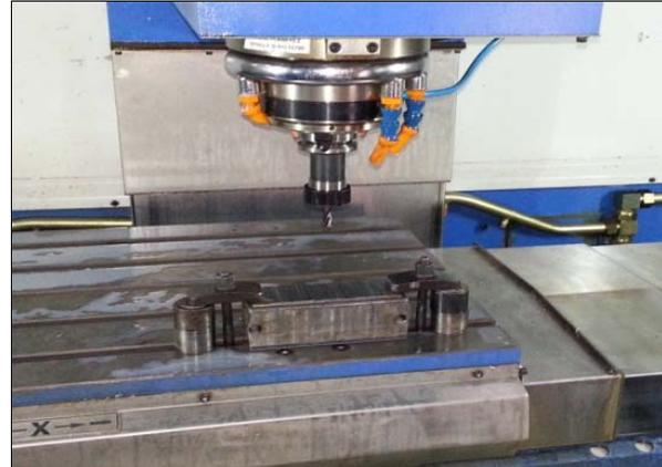
**Figure-1(a).** Experimental set up for end milling operation.
