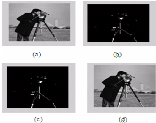
Figure-2. (a) Original image, (b) Scrambled images, (c) Encrypted images with message (d) decrypted version.
