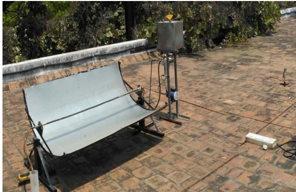
Figure-1. Solar parabolic trough collector.
