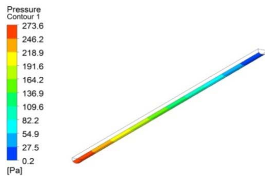
Figure-17. Pressure drop profile of the absorber tube with semi circular insertion.
