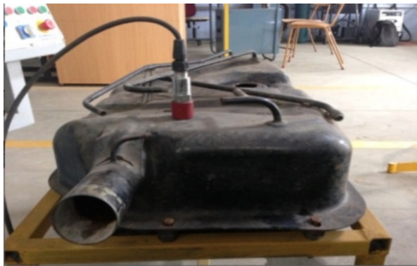
Figure-7. Experimental setup - fuel tank with accelerometer
