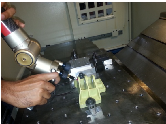
Figure-8. On machine capture of points by probe.
