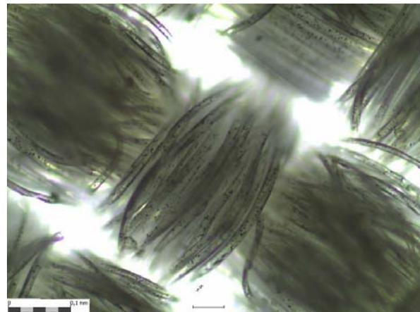
**Figure-7.** Polyester fabric with impregnated particles.
