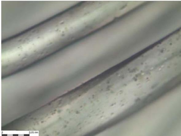
Figure-2. NaOH treated polyester fiber.
