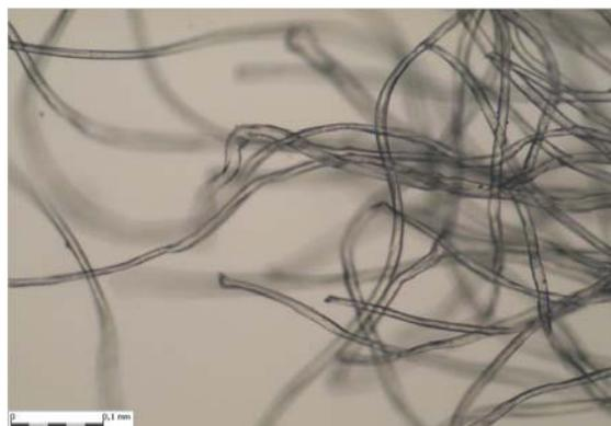
**Figure-1.** Optical microscopic image of polyester fiber.
