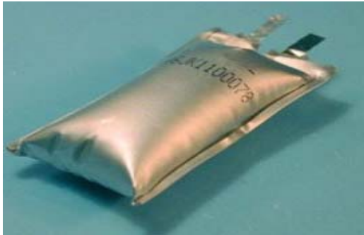
Figure-3. Swelling can occur as part of gas generation. The reasons for that are still not fully understood. Courtesy of Cadex [12].
