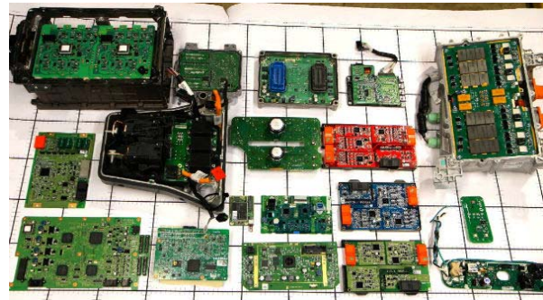
Figure-9. The battery-interface control module is composed of the red, blue, and green boards shown above in the second column from the right. (Courtesy of UBM TechInsights).
