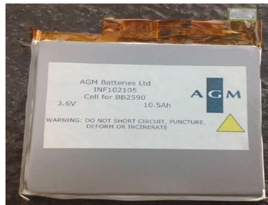
Figure-1. The pouch cell offers simple, flexible and lightweight solution to battery design. Exposure to high humidity and temperatures shorten service life. Courtesy of Cadex [12].
