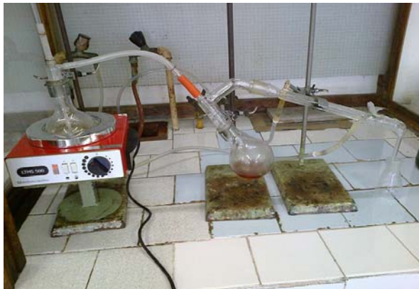
Figure-2. Apparatus for steam distillation.
