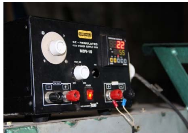
Figure-10. Electronic control unit for semi automatic system batik printing.
