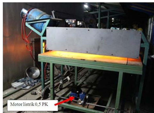
Figure-11. The dryer box of semi automatic system batik printing.
